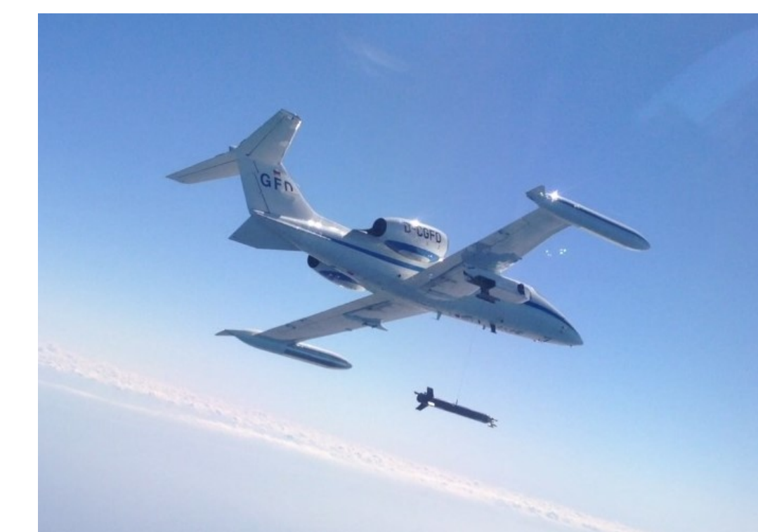
Figure 6: Measurement platforms for TPEX II – Learjet and TPC-TOSS
