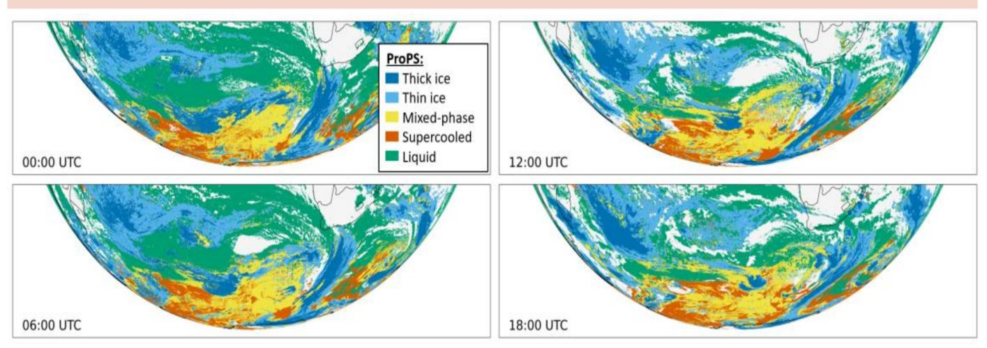
A short time series (00, 06, 12, 18 UTC) of cloud top phase evolution on 01.01.2022 over the Southern Ocean derived with the MSG retrieval ProPS.
